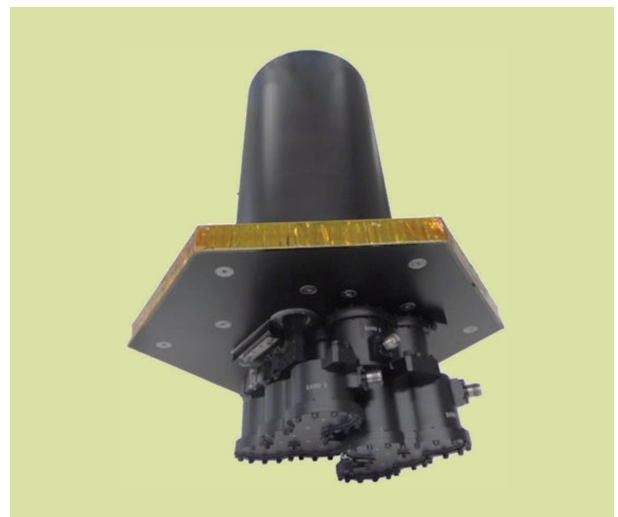
FIGURE 14. An integrated radiating element with a low-loss triplexer.
