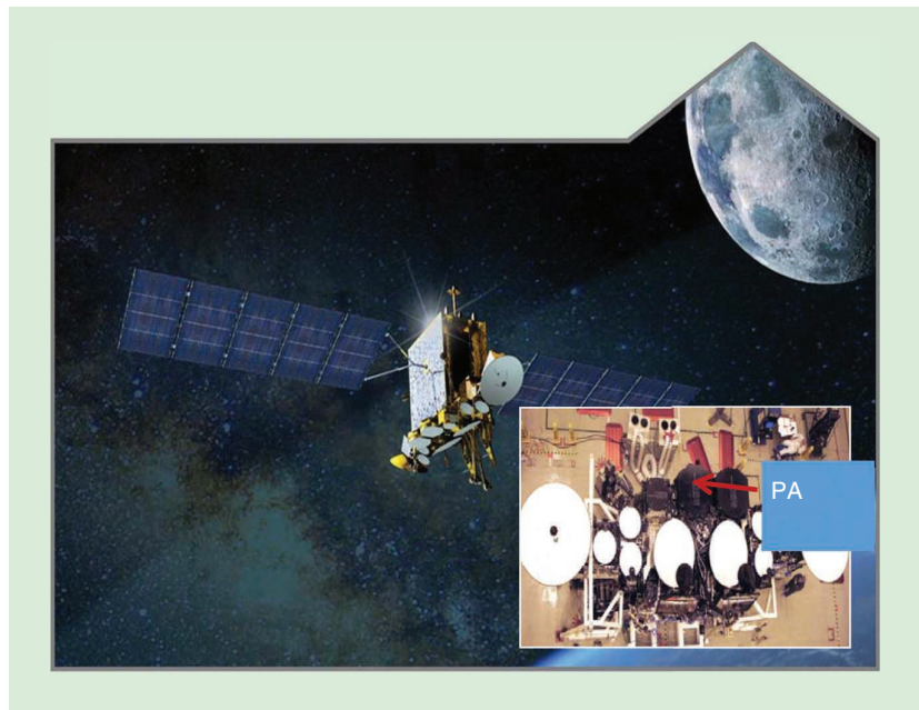
FIGURE 1. An AEHF satellite with multiple PAs and reflector antennas. The inset shows various antennas deployed. (Source: Northrop Grumman Aerospace Systems; used with permission.)
