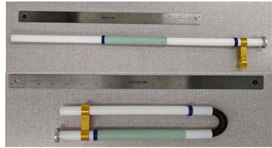
Fig. 5. Fabricated RMA prototype showing deployed (top) and stowed (bottom) configurations.
